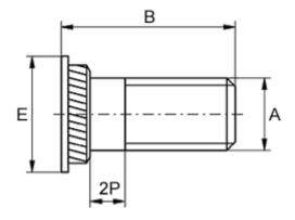
For plate thickness, min = 1.5 Head diameter E = 7 Hole diameter +0.1 = 6.4 Length B = 15 Male thread A = M4x0,7 Min distance to edge = 3.3
